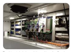
The integrated design, which combines the fiber laser generator and chiller with the machine frame, allows for shipment after factory testing without the need to disconnect these key components from the machine. Installation and start-up time is reduced from weeks to days compared to conventional laser cutting machine designs.
