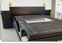
It has two dynamic tables allowing continuously production while processing goes on. The operator collects cut parts and loads the next material for processing. Fully automated loading – unloading systems.
