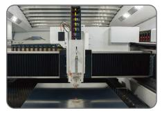
The fiber laser adds faster cutting speeds, the ability to cut a wide-variety of material types and reduced operational costs which add to a company's profit margin.
